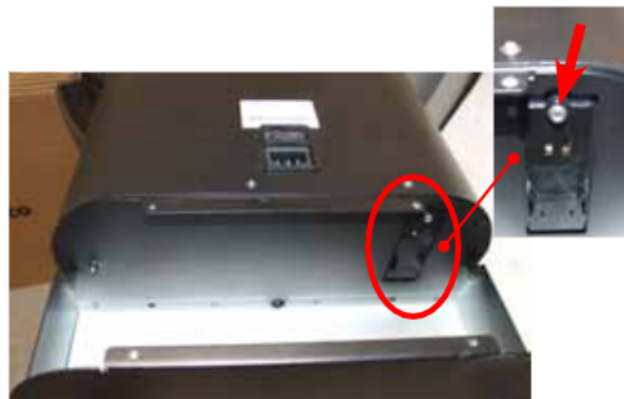
Loosen the screw shown in the picture and remove the back panel
