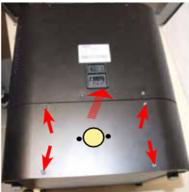
Loosen the screws shown in the picture and remove the back panel
